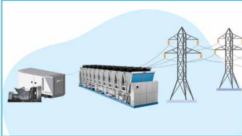
Dual power back-up for non-stop running of the chiller controller
